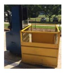
Hydraulic lift boarding device platform to carriage
